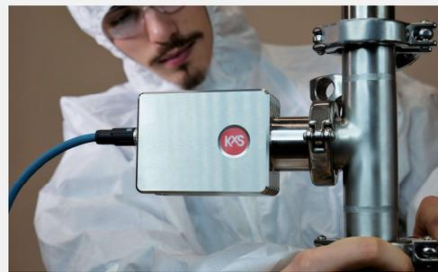
The DCM-20 inline Brix monitor is mounted to a single-piece flow cell SFC exceptionally machined out of one metal block without welding joints to ensure surface finishing quality. The sensor and flow cell wetted parts are of stainless steel 316L. The flow cell dimension is scalable for mounting in corresponding **1", 1.5", 2", 2.5", 3" or 4" process line sizes**.
