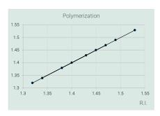
The refractive index curve shows a steady linear increase corresponding to the degree of polymerization. When the reaction achieves the endpoint the refractive index curve levels off.
