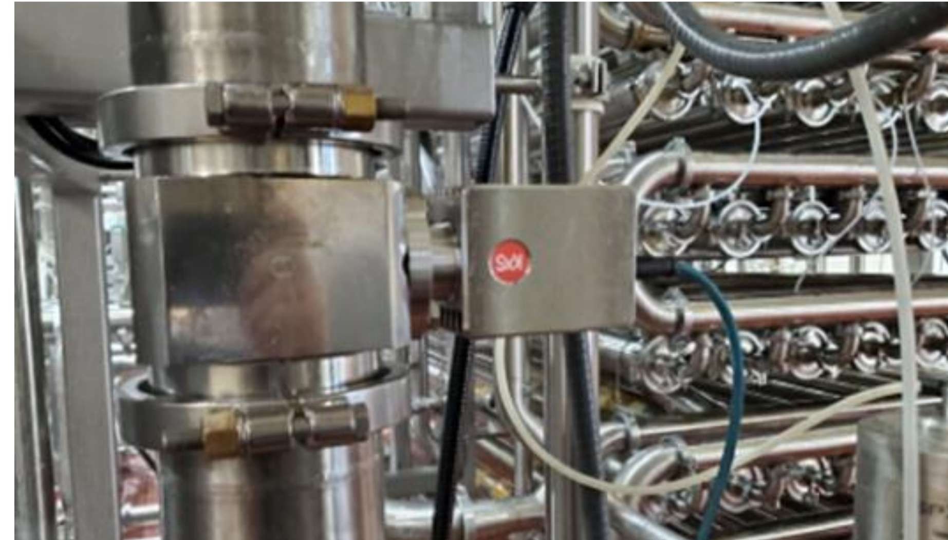
Inline refractometer in membrane filtration
