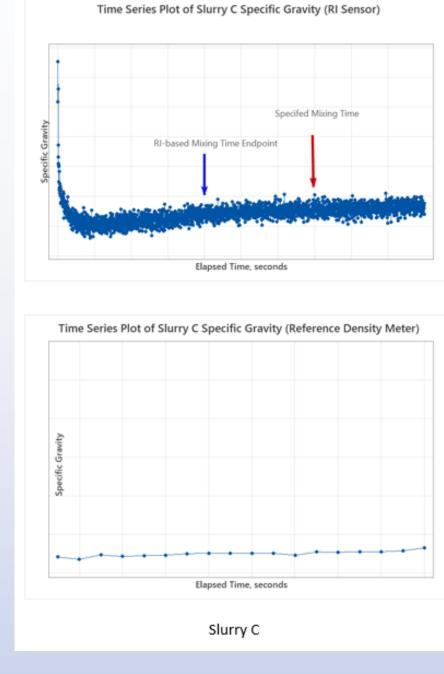
The results effectively demonstrate that the dispersion of raw CMP slurries can be effectively characterized by the KxS RI sensor. Incorporating the feedback system to manage the dispersion time based on the RI sensor's output signal provides a real-time health indicator of the raw slurry under dispersion. This data-driven approach would be a viable option for process and operational improvements for Fab Facilities Operations teams.
