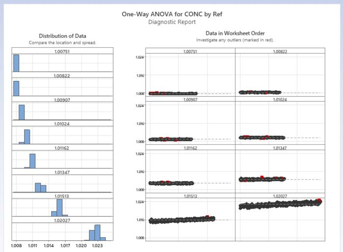
The RI sensor was less susceptible to pump flow and pressure fluctuations versus the reference metrology. The charts below shows the comparison of the possible mixing time reduction of CMP Slurries A, B and C based on the RI-based trend versus the fixed mixing time as per initial specification. Mixing Time Endpoint is achieved once stable density/specific gravity reading (+/- specified control limits) is monitored for a given window period.
