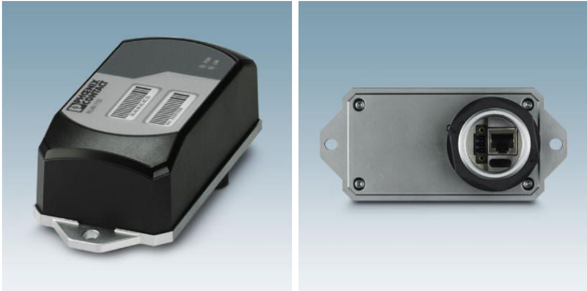
Figure 32 WLAN access point, client with two internal antennas (MIMO) for single hole mounting, IP54, WLAN 802.11 a, b, g, n, frequency: 2.4 GHz, 5 GHz (incl. DFS channels), connections: COMBICON 9 ... 32 V DC, RJ45: for LAN, web, http/https, Command Line Interface.
