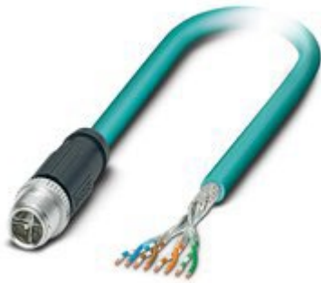
Figure 36 Network cable, Ethernet CAT6A (10 Gbps), CC-Link IE CAT6A (10 Gbps), 8-position halogen-free, shielded (Advanced Shielding Technology), Plug straight M12 / IP67, coding: X, on free cable end, coding: X
