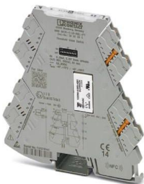
Figure 37 Limit value switch with changeover relay output for monitoring analog limit values from the sensor output. The sensor wash is activated at a mA value that corresponds to the limit value switch schedule with DIP switches activated. The relay closes or opens per user selection.
