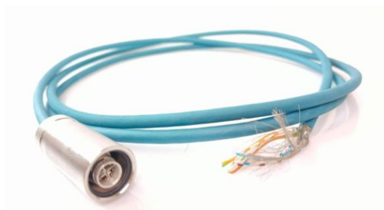
Figure 9 Network cable with connector cover 10318 attached (Material 1.4404), Ethernet CAT6A (10 Gbps), CC-Link IE CAT6A (10 Gbps), 8-position halogen-free, shielded (Advanced Shielding Technology), Plug straight M12 / IP67, coding: X, on free cable end, coding: X.
