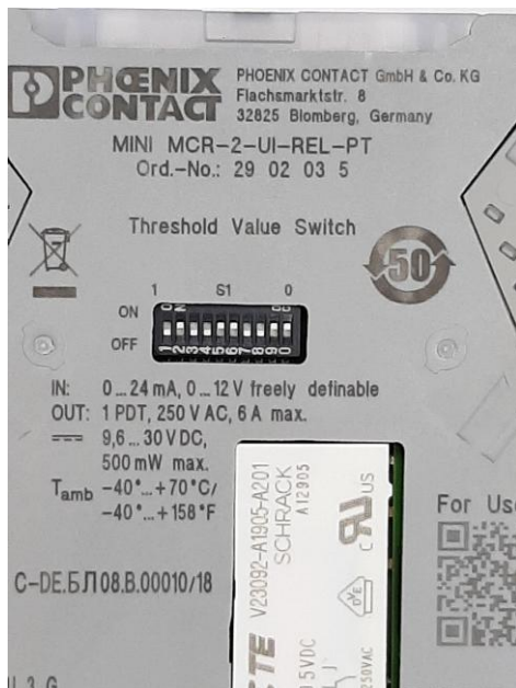
Figure 49 Physical DIP switch configuration for Low alarm functions. DIP switches 3, 5, 6, 9, 0 activated 'ON'
