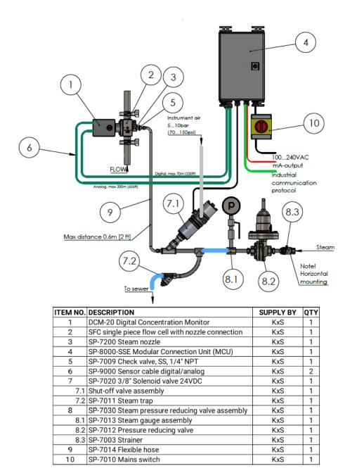
Figure 19 DCM-20 steam wash system. DWG No. 10467.
