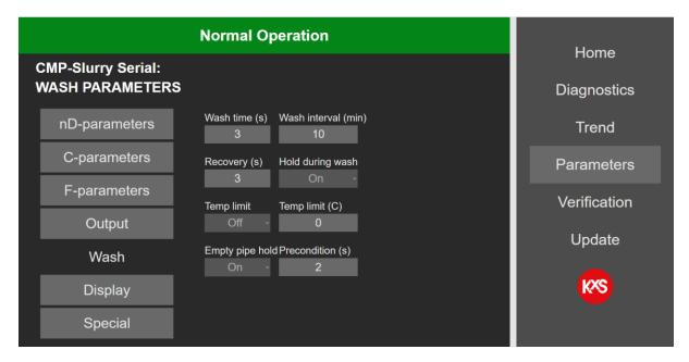
Figure 35 Optical window wash function and time settings.
