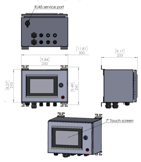
Figure 39 Dimensional drawing of Modular Connection Unit enclosure DWG No. 10528.
