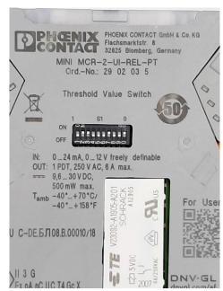
Figure 34 Physical DIP switch configuration for High alarms functions. DIP switches 3, 7, 0 activated 'ON'
