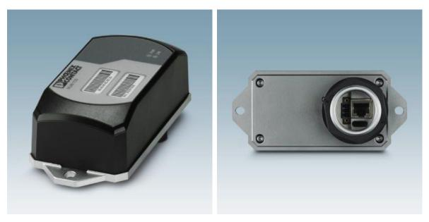
Figure 41 WLAN access point, client with two internal antennas (MIMO) for single-hole mounting, IP54, WLAN 802.11 a, b, g, n, frequency: 2.4 GHz, 5 GHz (incl. DFS channels), connections: COMBICON 9 ... 32 V DC, RJ45: for LAN, web, http/https, Command Line Interface
