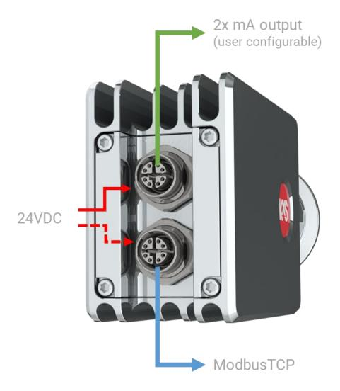
Figure 1 DCM-20 inline optical Brix monitor connectors
