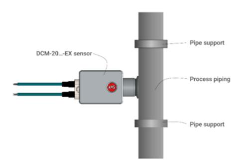
Wall thickness between sensor process side to electronic compartment is 1.5mm stainless steel, Nickel, Hastelloy or titanium. The DCM sensor sapphire measurement window thickness is 8mm.
