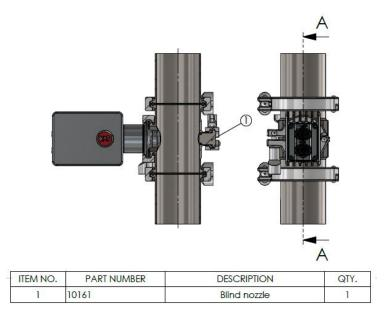
Figure 16 Blind nozzle insert when wash nozzle not mounted. DWG No. 10164.
