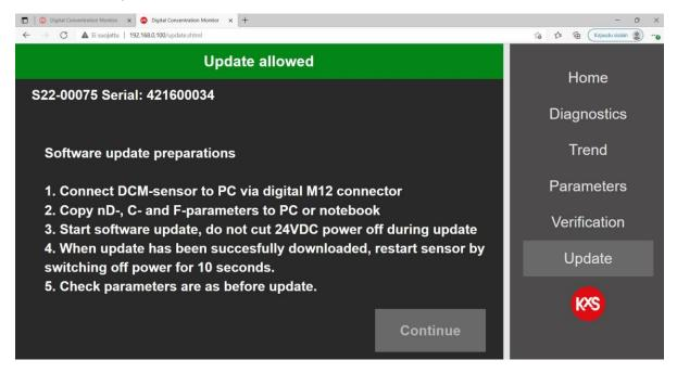
Figure 37 Guided sensor software procedure
