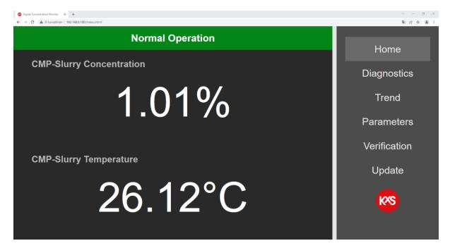
Figure 23 User interface homepage with real-time measurement values.
