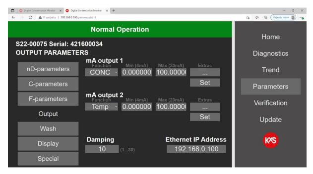
Figure 31 User configurable analog measurement output settings.
