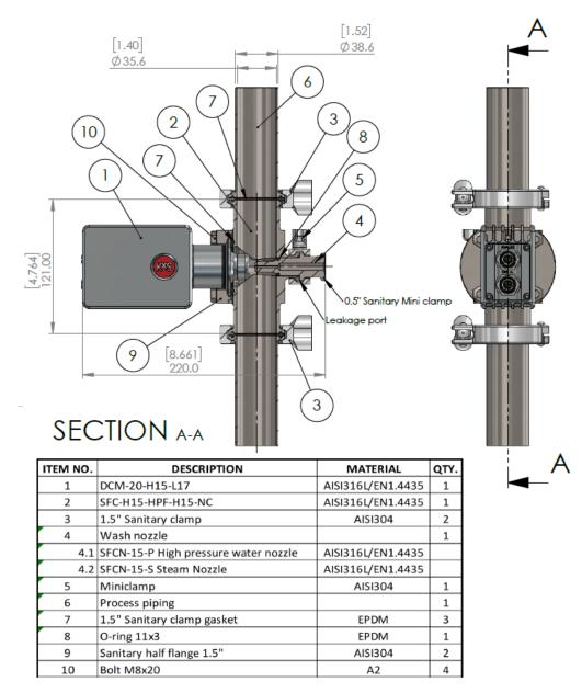
Figure 15. Sensor mounting in single-piece flow cell with optional wash nozzle. DWG No. 10288.
