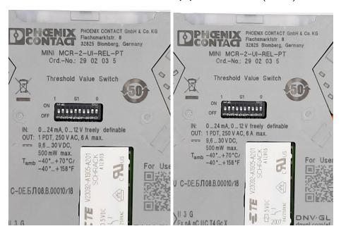
Figure 21 DIP switch configuration
