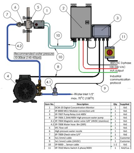
Figure 18 DCM-20 High pressure water system. DWG No. 10177-C.
