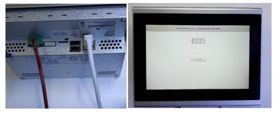
Figure 9 Cable connections to the external display and activation of configuration page during power up.
