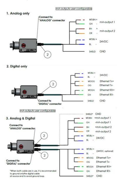
Figure 2 Inline Brix monitor DCM-20 operation concept. DWG No. 10125.
