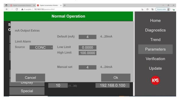
Figure 32 User selectable alarm limit function.
