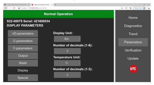
Figure 36 Displayed engineering units for concentration and temperature.
