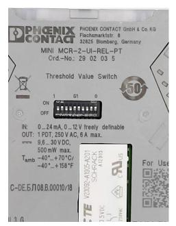
Figure 33 Physical DIP switch configuration for Low alarm functions. DIP switches 3, 5, 6, 9, 0 activated 'ON'
