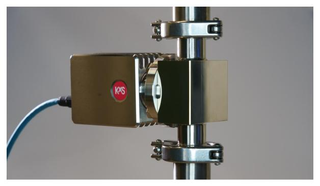
Figure 13 Inline optical Brix refractometer mounted in process pipe.
