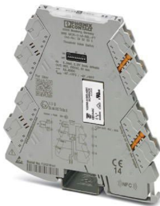
Figure 48 Limit value switch with changeover relay output for monitoring analog limit values from the sensor output. The sensor wash is activated at a mA value that corresponds to the limit value switch schedule with DIP switches activated. The relay closes or opens per user selection.
