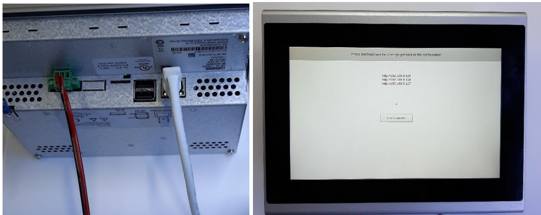
Figure 15 Cable connections to the external display and activation of configuration page during power up.
