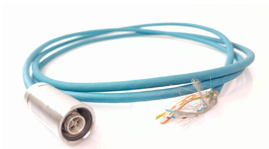
Figure 5 Network cable with connector cover 10318 attached (Material 1.4404), Ethernet CAT6A (10 Gbps), CC-Link IE CAT6A (10 Gbps), 8-position halogen-free, shielded (Advanced Shielding Technology), Plug straight M12 / IP67, coding: X, on free cable end, coding: X.
