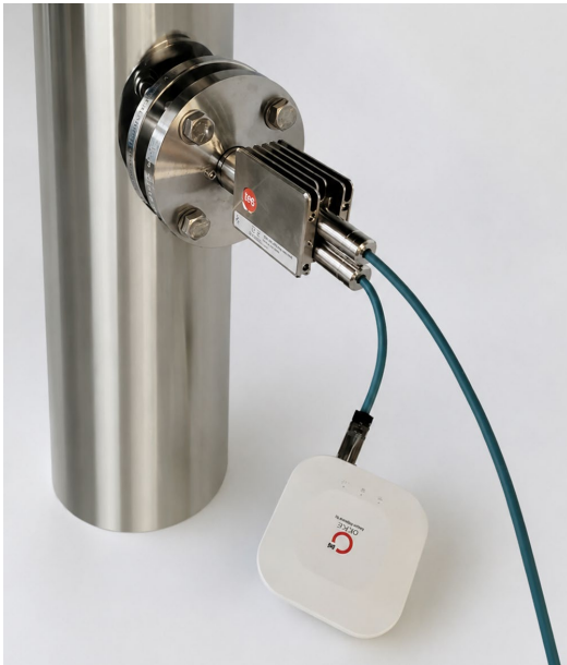
Figure 19 Portable 4G/LTE WiFi router connected to the DCM-20 refractometer for wireless access.
