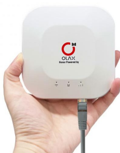
Figure 18 Example of a portable 4G/LTE WiFi router used for wireless access to the DCM-20 refractometer.
